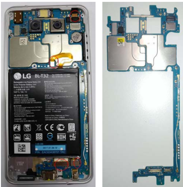
7. Disconnect 4 connectors / main PCB
