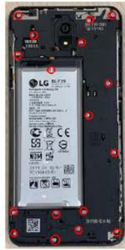
6. Disassemble HW Parts (2ea)
