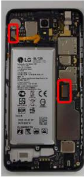
5. Disassemble Connector (2ea) and Main PCB
