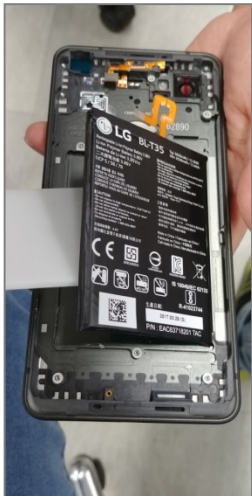
17. Lifts up the battery using the hera
