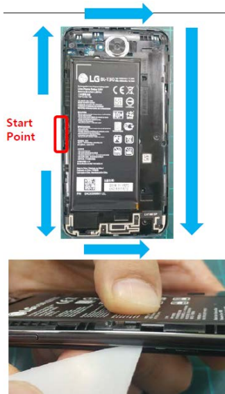
5. Insert the disassembly tool into rear
