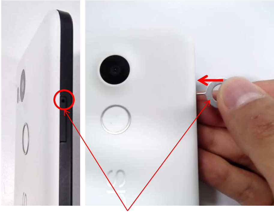
Using SIM ejection, remove SIM tray
