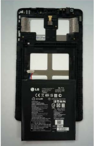
Disassemble battery pack by tool. (The principle of the lever)
