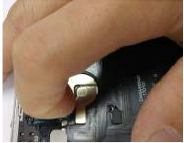
6. Disassemble rear cover
