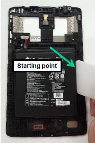
Disassemble battery pack by tool. (The principle of the lever)
